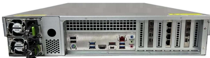
Rear (full option): two hot-swappable redundant AC PSU modules · I/O panel · expansion slots
