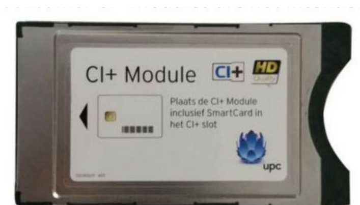
Figure 4.1 A consumer CI+ module: up to two services in parallel. Product photo: third party
