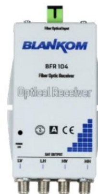
Figure 6.5 BFR-11 compact optical receiver (o/e), powered from the multiswitch – no own power supply. The picture shows the earlier model label.
