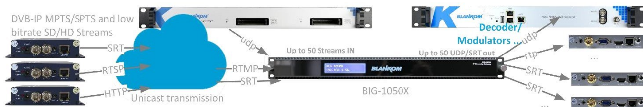
Figure 17.3 BIG-1050X converting SRT, RTSP, RTMP, HTTP and UDP streams, unicast and multicast, for decoders and modulators.
